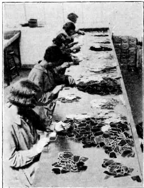
Precision work at Messrs. Dubilier's factory—measuring the thickness of small sheets.
