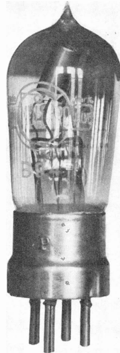
Fig. 10.—The D.F. ORA has inclined electrodes which distinguish it from the ordinary ORA.
