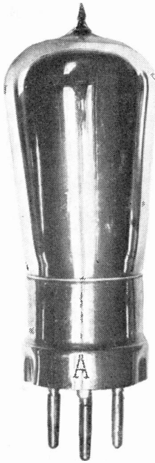
Fig. 9.—The construction of the B.5 is obscured by the magnesium getter.
