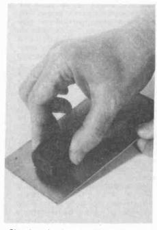
Cleaning the board with an abrasive block.
