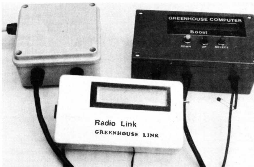
The three modules that make up the Greenhouse Computer, (left to right) mains power unit, radio link and greenhouse controller.
