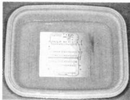
Exposed p.c.b. immersed in developer to remove unwanted resist.
