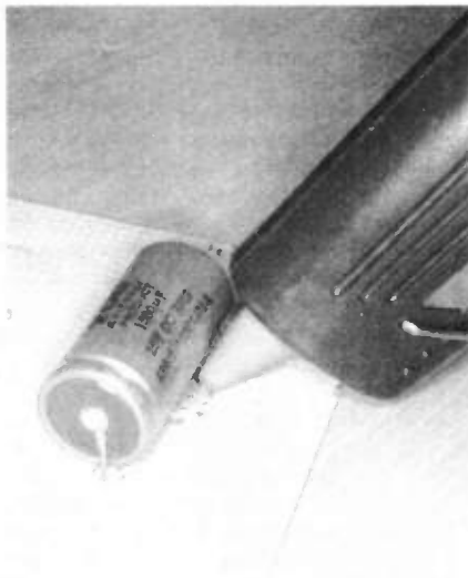
"Hot-melt" glue is useful for protecting larger parts from breaking loose due to vibration.
