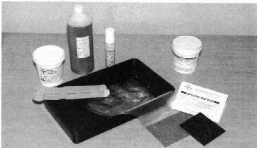
Materials needed for developing and etching printed circuit boards: Ferric Chloride crystals, developer, photoresist, caustic soda, plastic tongs, plastic tray, disposable gloves and photoresist copper board.
