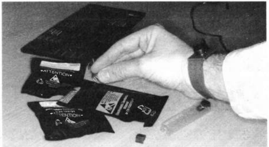
Anti-static wrist-strap is preferable when handling CMOS devices.
