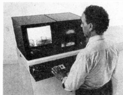
Modular Vision computer which relays the X-ray pictures.
