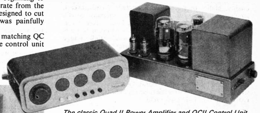
The classic Quad II Power Amplifier and QCII Control Unit. Manufactured unchanged for 18 years.
