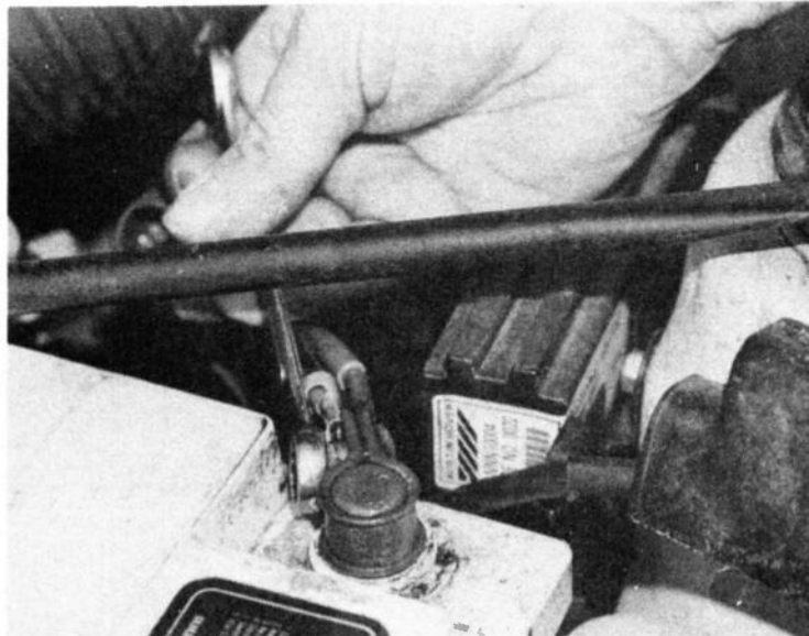
When tightening the battery positive clamp, the spanner MUST NOT TOUCH ANY METALWORK – see text.
