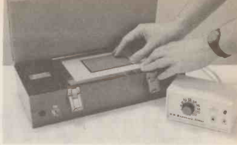
Photo 3. Aligning the sensitive p.c.b. with the artwork, on an ultra-violet light unit. The EE UV Exposure Timer, to be described next month, is adjacent.
