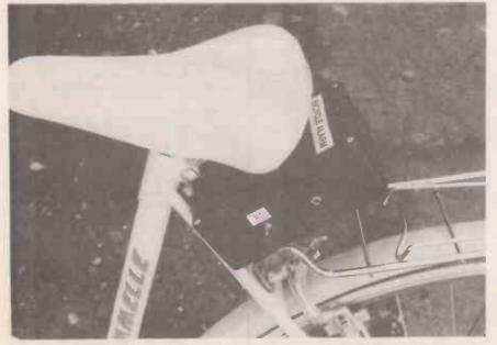
This unit is attached to the bike frame with two Jubilee clips bolted to the case. This is the suggested position for the finished unit.
