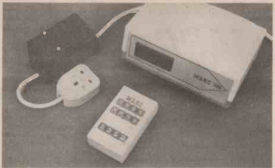
The completed decoder, encoder and infra-red transmitter.
