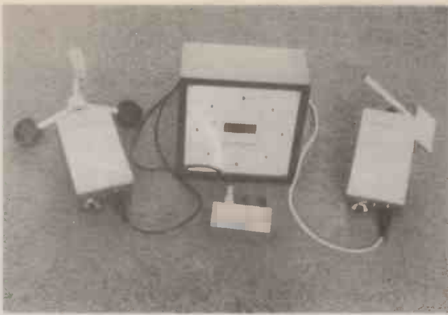
The three sensor heads plugged into the rear of the display cabinet.
