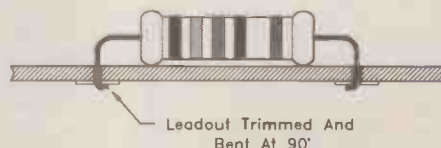
Fig. 2. By cutting and kinking lead-out wires, a special wire cutting tool fixes components in position.
