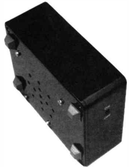
Bottom and side view of completed unit showing speaker "grille", rubber feet and on/off switch.
