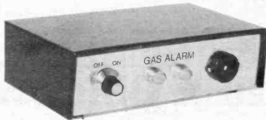
(Left) Rub-down lettering applied directly on the front panel, prior to final mounting of components. Gas Alarm (Aug '92).
