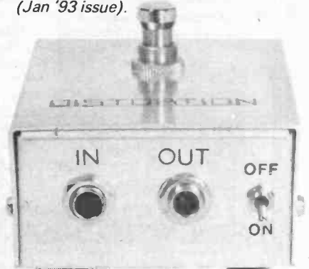
(Below) Black rub-down lettering applied directly on the aluminium box and covered with protective, clear varnish - Soft Distortion Unit (Jan '93 issue).
