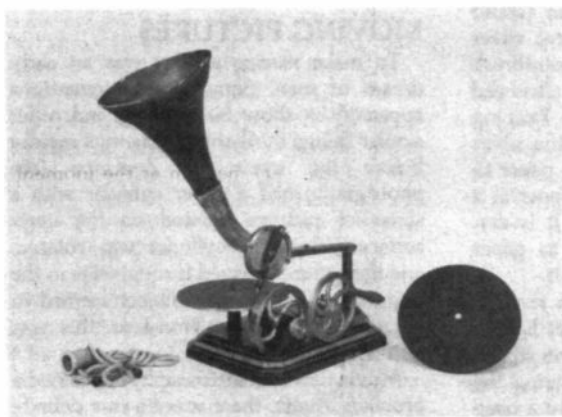
Berliner disc gramophone (1890) (Reproduced by permission of the Trustees of the Science Museum)
