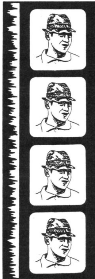
Fig. 2. An optical sound track running down the side of a film.
