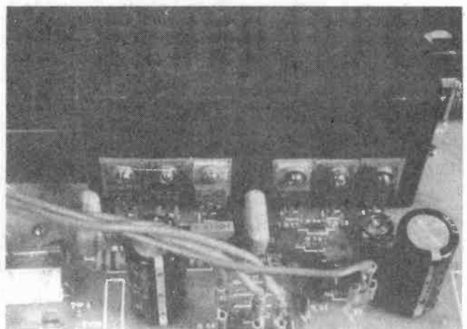
The speaker leads attached to the board "spade" terminals. Also note the insulating washers behind the transistors.
