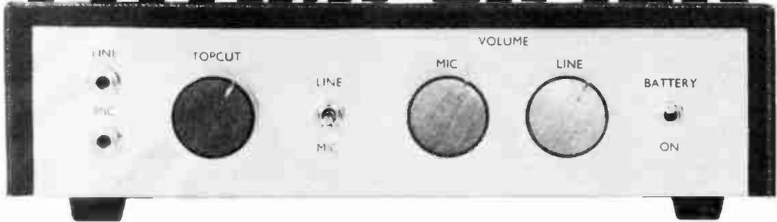
Twenty watts r.m.s. for around £20. Designed for the home constructor using just three i.c.s and a handful of discrete components. This unit is capable of a respectable performance while still being inexpensive to build.
