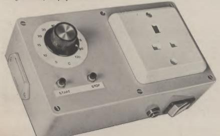
the mains. Meanwhile, the contacts of RLA short-circuit the "start" switch, S2. Thus, when S2 is pressed for an instant, the i.c. will be triggered by the pulse of charging current to C2 taking pin 2 low. The contacts of RLA then "take over" from S2 in allowing battery current to flow until the end of the timing cycle. Timing may be interrupted at any time by momentary breaking of battery current by means of S3 which is a push-to-break switch.
