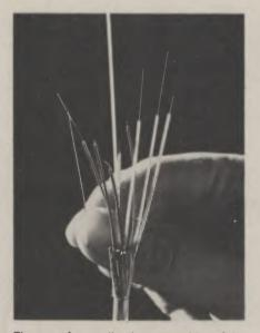
The eye of a needle gives some idea of the scale of a typical optical fibre cable.
