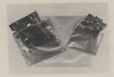
Anti-static packaging for circuits that include static-sensitive devices.
