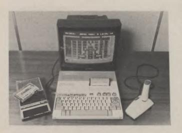
The Hitachi H-1 model MSX microcomputer on which will be based the MB-H80 family computer for the UK market.
