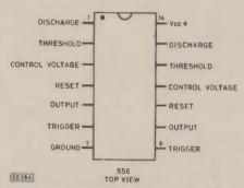
Fig. 2.15. The 556 i.c. comprises two 555s in a single package.
