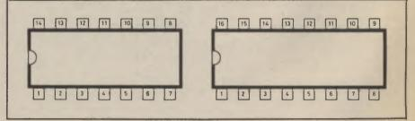
Fig. 2. Dual-in-line 14-pin and 16-pin TTL i.c.s have a notch at the end of the package to identify pin 1.
