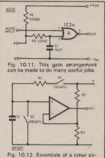
rig. 10.12. Essentials of a timer circuit. Closing S1 allows C1 to charge via R1. Closing S2 discharges C1 and so resets the circuit. In timer i.c.s the functions of S1 and S2 are performed electronically. It's good practice to connect unused inputs permanently to the + or - line to avoid the possibility of stray voltages getting to them.
