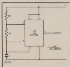
Fig. 2.2. The basic oscillator circuit for the 555 and the ICM7555.
