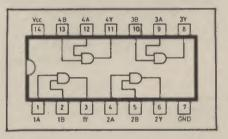
Fig. 3. Internal connections for a 7408 or 74LS08 quad 2-input AND gate.
