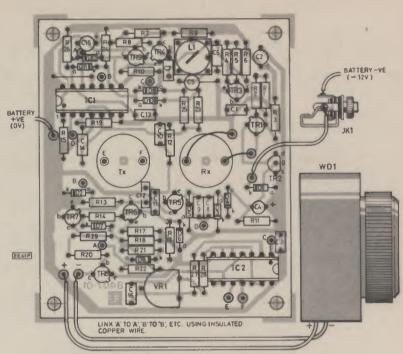
Fig. 3. Actual-size master pattern for the Ultrasonic Burglar Alarm. This board is available from the *EE PCB Service*, Order code 8407-01.
