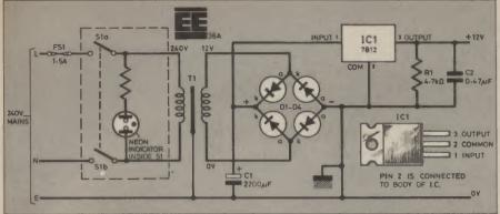
Fig. 1. Complete circuit diagram for the CB Mini PSU.
