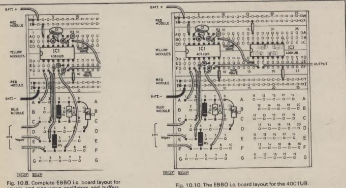
Fig. 10.8. Complete EBBO i.c. board layout for square and sine-wave oscillators and buffers, Fig. 10.6 and Fig. 10.7, respectively.
