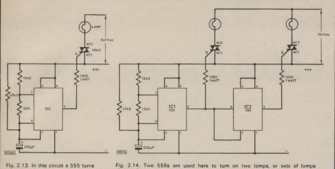
Fig. 2.13. In this circuit a 555 turns on a triac when its output is low.
