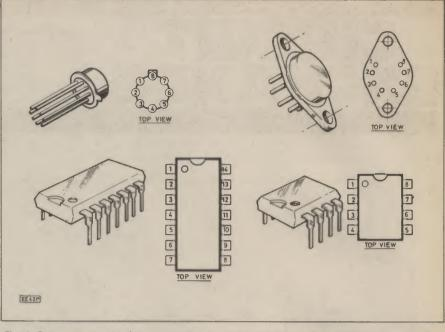
Fig. 1. Pin numbering for llnear i.c.s. Metal cans have either a tag or a wider pin spacing to identify pin 8. Dual-in-line packages have a notch and/or a depression to indicate pin 1.
