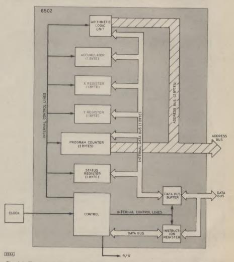
Fig. 1.1. The main sections of the 6502 microprocessor. Arrowheads indicate direction of control, or flow of data.
