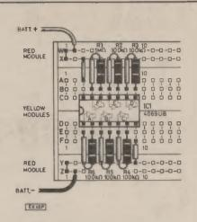
Fig. 10.5. EBBO i.c. layout for biasing experiment. The positions of the six inverters are shown on IC1 outline.
