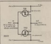
Fig. 10.3. CMOS inverter as contained in the 4069UB i.c. (Numbers refer to 4069 pins.)
