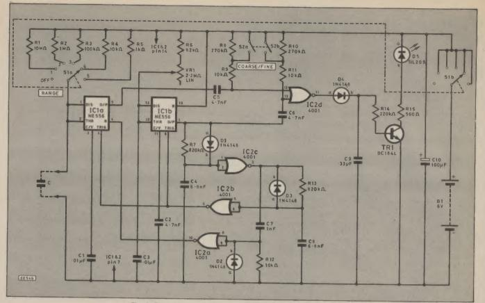
Fig. 1. Complete circuit diagram of the Capacitance Comparator.
