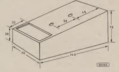
Fig. 5. Case dimensions. The circuit board stands 18mm off the panel, screwed onto pillars of wood, or bolted using spacers.
