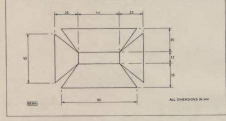
To save the cost of a key on-off switch a 2.5mm jack socket is proposed; the unit is switched off by inserting the jack plug. Front panel cut out and drilling dimensions are shown for the box proposed in the parts list. If the relay is used instead of the sounder, no hole is required and the relay may be glued to the sounder position. The relay coil is connected to the alarm output and the relay contacts may be brought out through a DIN connector, or jack plug and socket.
