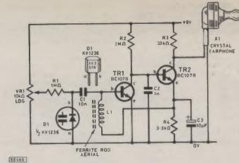
Fig. 9.5. Simple a.m. radio. L1 is the ferrite aerial winding and is tuned by variable capacity diode D1.
