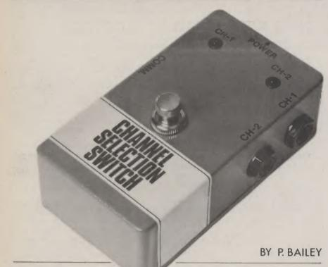
N RECENT years a large number of musical instrument amplifiers with two input channels have been fitted with a facility which allows the performer, via a footswitch, to electronically switch between the two channels. This eliminates the need to alter controls on the amplifier or unplug leads, something which can be difficult on a dimly lit stage.
