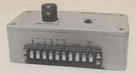
the case can be drilled to accommodate fixing screws with which to mount the unit on the control panel. The layout of the unit is shown in the accompanying photographs.
