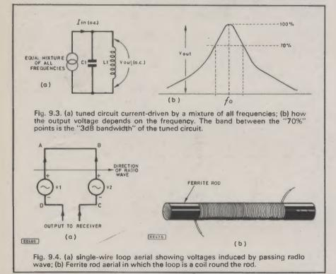
voltage (V1) in AD and V2 in BC. Nothing is induced in AB and DC because these wires are end-on to the wave so it cannot "see" them.
