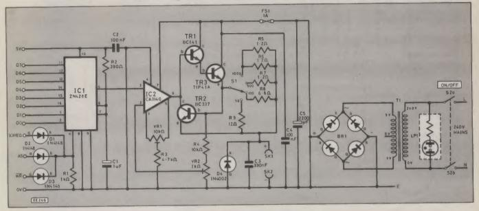
address 65503. There are in fact other addresses which could be used, but 65503 is the best one as it does not take any of the other address lines low and will not interfere with any of the Spectrum's internal input/output circuits.
