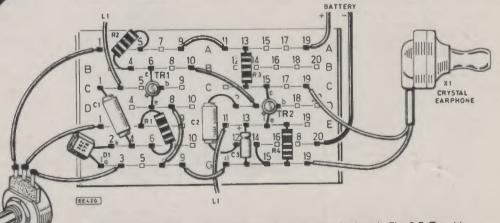
Fig. 9.6. The EBBO discrete board layout for radio circuit given in Fig. 9.5. To add the reaction circuit, Fig. 9.7, remove the link between D8 and G7 and replace it with potentiometer VR2; connect L2 between D4 and G5.
