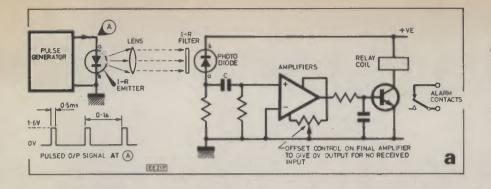
Fig. 2. (a) Infra-red beam fence arrangement. (b) Infra-red transceiver. The first amplifier is offset to give OV output for OV input.
