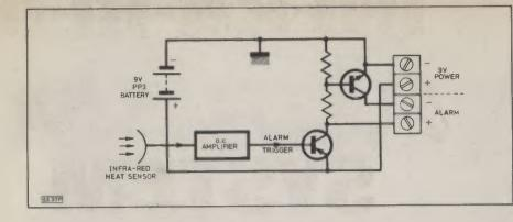
Fig. 1. Infra-red sensor unit internal circuitry.
