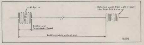
Fig. 6. Time scale for transmission and reception of ultrasonic pulse.
