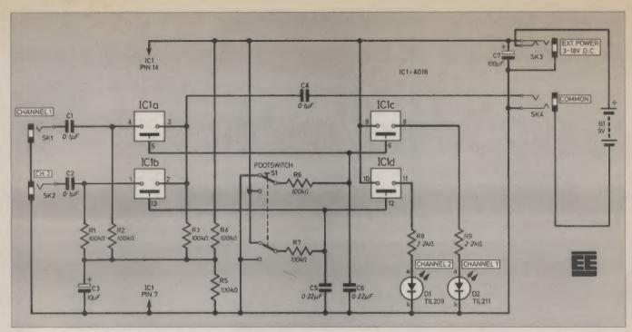
Fig. 1. Circuit diagram of the Channel Selection Switch. Note the insertion of a mono plug into stereo socket SK4, switches the unit on.
