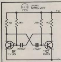
Fig. 1.3(a). A multivibrator with a calculated frequency of 984Hz.
