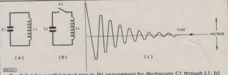
Fig. 9.2. (a) a parallel-tuned circuit; (b) arrangement for discharging C1 through L1; (c) how the voltage behaves after S1 is closed.
