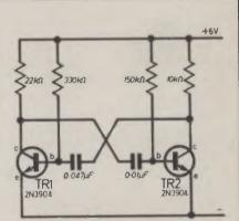
Fig. 1.4. With this multivibrator the transistors are turned off for different lengths of time during the cycle.
