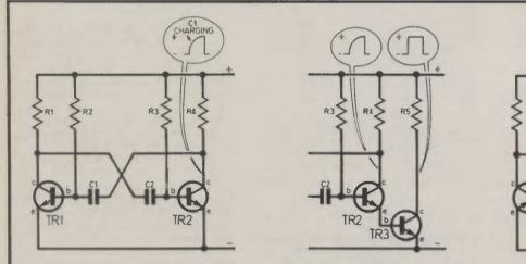
Fig. 1.8. Adding a third transistor, TR3, allows pulses with sharp leading edges to be produced. Because of the current gain provided by TR3, R5 can if desired have a much lower value than R4.
