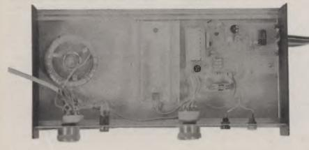
A hole for the mains lead should be drilled in the rear panel, and this should be fitted with a grommet to protect the cable. Using the specified case the ribbon cable can be taken through the gap between the base panel of the case and one of the side panels, but obviously it will almost certainly be necessary to cut or file out an exit hole for the cable if a
