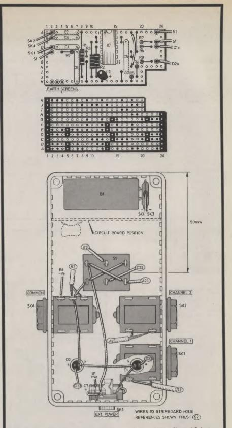
Fig. 2. Circuit board layout and case assembly diagram for the Channel Selection Switch. Interwiring details are also given and note that the OV connection to the board is made via the earth screens of the screened cables from SK1, SK2 and SK4. The position of the board is shown dotted and a piece of cardboard must be placed between the board and the battery, B1.
