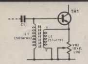
Fig. 9.7. Add-on "reaction" circuit.
