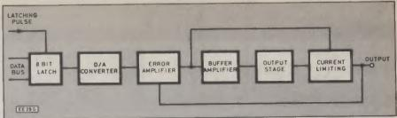
Fig. 2. Block diagram of the Bench p.s.u.
