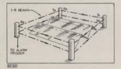
The two systems are illustrated in the simplified block schematics of Fig. 2 together with a diagrammatic illustration of an infra-red emitting diode and photodiode detector (Fig. 3).
