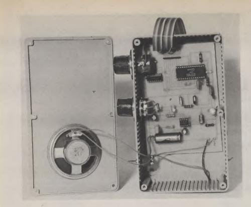
The completed Speech Synthesiser model with cover removed to show positioning of circuit board and control potentiometers. The speaker is mounted on the rear of the lid of the case.
