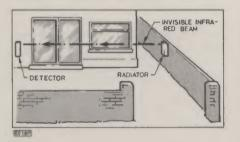
Fig. 1. Two infra-red beam break intrusion detectors.
