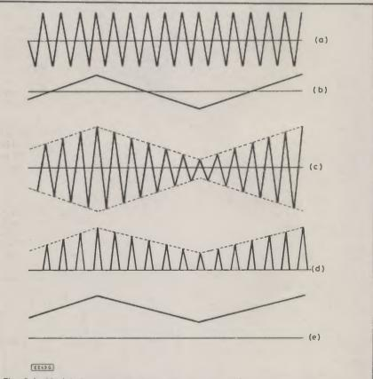
Fig. 9.1. Modulation and detection. (a) unmodulated carrier wave; (b) audio wave; (c) amplitude modulated wave when audio is made to vary the carrier amplitude; (d) half-wave rectified version of (c). This can be regarded as a sequence of samples of the original audio wave, (b); (e) smoothed version of (d) contains both audio and a d.c. component.
