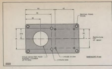
Fig. 5. Lid drillings. A cardboard template should be made first, so that the lid can be centrepunched without having to deface it with markings. Right: The complete system In situ.
