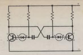
Fig. 1.6(a). Problems with base-emitter breakdown voltages can be removed by inserting small silicon signal diodes, as here
