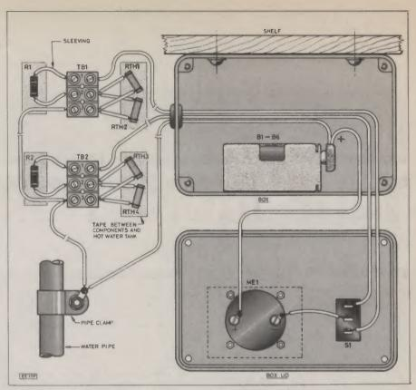
Fig. 2. Method of mounting thermistors in terminal blocks and interwiring to battery, meter and temperature switch S1. The battery holder contains six HP7 cells.
