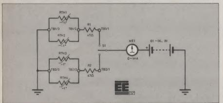
Fig. 1. Circuit diagram for the Hot Water Tank Indicator.
