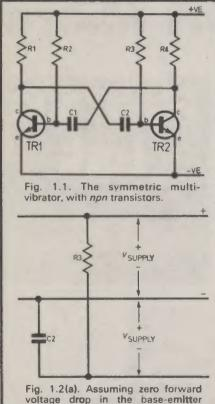
voltage drop in the base-emitter junction of TR2, the voltage conditions at the instant when TR1 turns on are as shown here.
