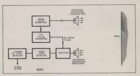
Fig. 7. Block diagram of ultrasonic transceiver.
