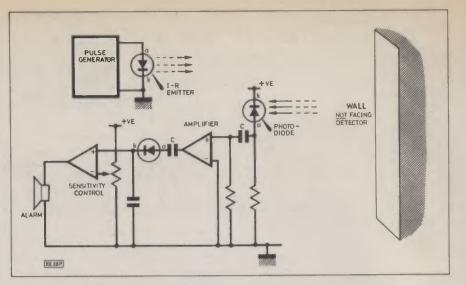
Fig. 4. IR proximity detector.
