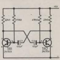
Fig. 1.3(b). The cycle length of this multivibrator lies, in practice, between some 60 and 100 seconds.
