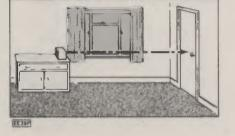
Fig. 5. An ultrasonic beam directed across a window will guard against an intruder entering via that window. If directed against a door it will also be disturbed by movement of the door. A beam aimed directly at a window, however, may give false alarms due to reflections from draughts of air at differing temperatures.
