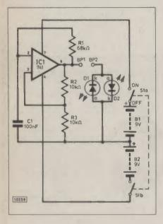
Most electronics experimenters seem to have plenty of diodes in their junk boxes, either salvaged from old units or purchased at low bulk prices. The problem is to find out which diodes are good, which are bad and in the case of the former, which end is which (cathode or anode).
