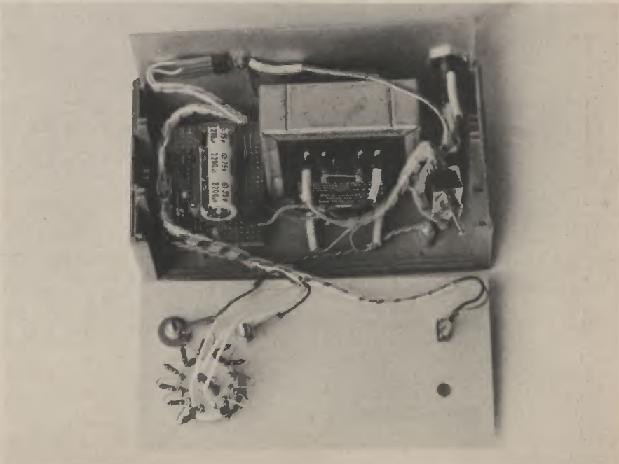
Fig. 2. The potential divider chain around S2. D6 establishes a reference voltage and points along the chain give voltages, that when multiplied by the gain of IC1 (set at 1.91 by R15 and R16), give the output voltages.
