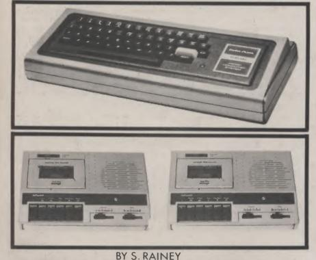
OWNERS of the TRS-80 Model I Level II Microcomputer will know that this computer has the capability of driving two cassette decks. However, with just the basic system, only one may be used, since only one I/O port is provided. On adding the expensive and now discontinued Expansion Interface, two cassette I/O ports are provided. This project provides two cassette ports for the basic system without the need for the Expansion Interface.
