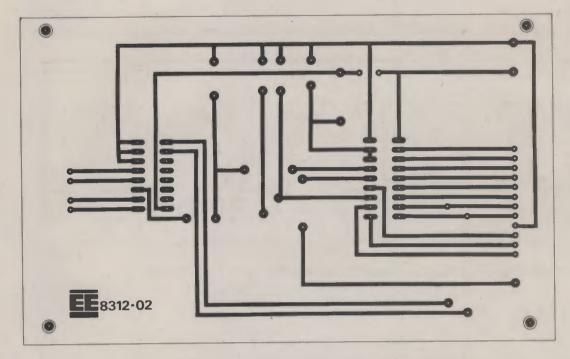
Fig. 6.8. Full-size printed circuit board master for the digital board.
