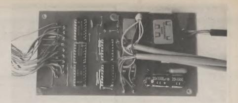
The complete prototype printed circuit board assembly.
