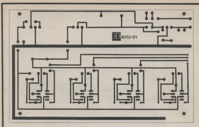
Fig. 6.6. Full-size printed circuit board master for the analogue board.
