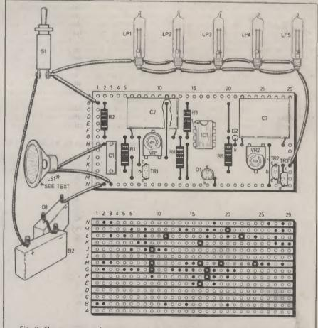
Fig. 2. The component layout and trackside view of the Disco Light's circuit board, with offboard wiring details also shown.
