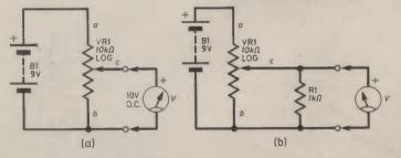
Fig. 3.3(a). How a potentiometer can "tap off' any portion of an input voltage. (Experiment 3.1); (b) Connecting R1 as a relatively low resistance "load" has a marked effect on the output voltage. (Experiment 3.2).
