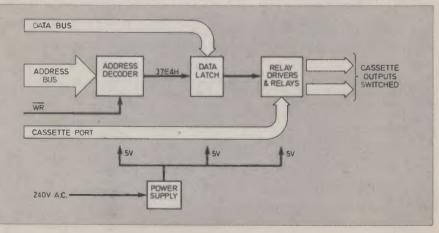
Fig. 1. Block diagram of the TRS-80 Twin Cassette Interface.
