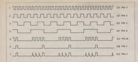
Fig. 3. Shown are the pulses that should be obtained when testing IC1, IC2 and IC3 with an oscilloscope. Note that pin 4 of the oscillator IC3 sees a full width pulse instead of a narrow pulse on the fourth count to produce the "squawk".
