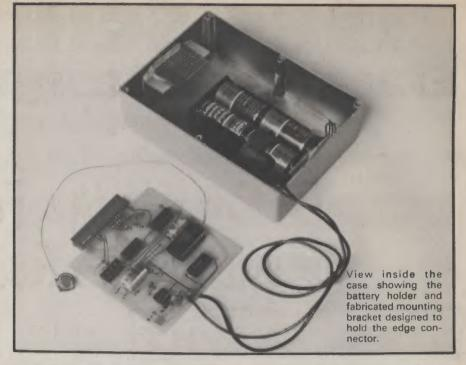
here uses less than 2mA compared with over 8mA in the original prototype unit presented for SEDAC. The timing circuit has been completely redesigned and the selection logic simplified.
