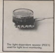
The last connections are the wires to the battery pack and to the sensor (on the prototype, a light dependent resistor, PCC1).
