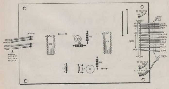
Fig. 6.9. Complete component layout for the digital (clock) board.
