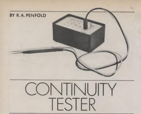
DESPITE the fact that a Continuity Tester is an extremely simple piece of test equipment it can nevertheless be very useful when fault-finding on electronic equipment. Uses of continuity testers include such things as checking fuses, tracing broken wires or printed circuit tracks, checking diodes, and tracing short circuits on printed circuit boards.
