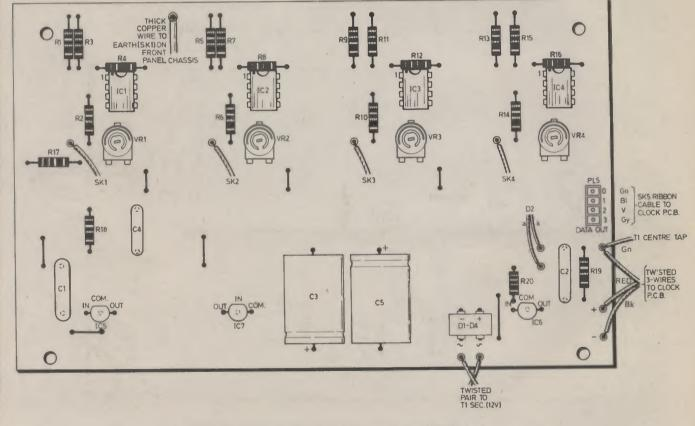
Fig. 6.7. Complete component layout for the analogue (ADC) board.
