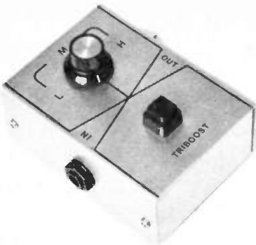
Topside of finished prototype showing the positioning of foot switch.
