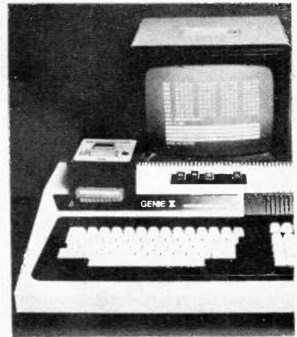
The Eprom Programmer in use with the Genie II microcomputer. The screen shows that a 4K-byte EPROM has just been successfully "burned".
