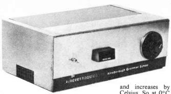
Completed prototype of the Beehive Temperature Meter. The frame selector switch is on the right and the remote sensor input socket can be seen on the side of the case.
