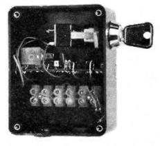
may be soldered into place and Veropins fitted where connections to off-board components are to be made. Take care with the CMOS i.c. since it may be destroyed by static.
