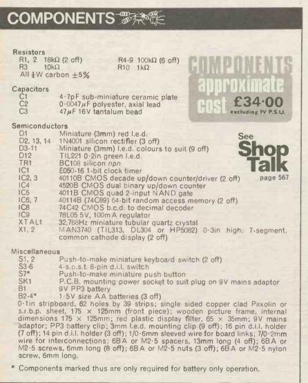
If the 9V adaptor voltage drops below 9V on load, a 1N4001 diode must be added in series with D13, effectively reducing the voltage at which the back-up battery is brought in.
