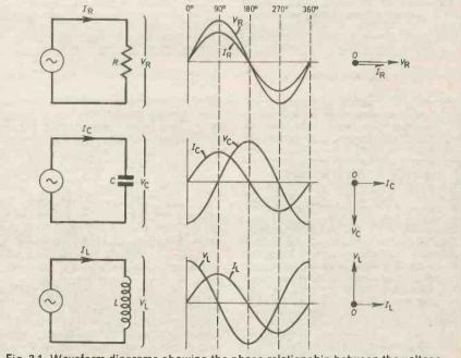
Fig. 3.1. Waveform diagrams showing the phase relationship between the voltage and current in a resistive circuit (top), a capacitive circuit (centre) and an inductive circuit (bottom). The phasor diagrams (right) illustrate this phase relationship. sum of the squares of the other two sides. So the resultant current,  $(I_2) = \sqrt{I_R^2 + I_L^2} = \sqrt{200} = 14.14$ A.
