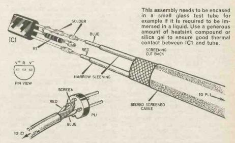
Fig. 9 Construction of the sensor assembly. The sleeving should be pushed over the soldered connections on IC1. It is important that the screening is not connected or in contact with the leads of IC1.
