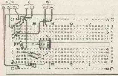
Fig. 12.7. The layout of the components on the Verobloc for the circuit in Fig. 12.6.
