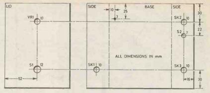
Fig. 6. Case drilling details.
