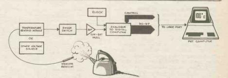
clocked into the chip to provide digital representation of the input voltage level in the form of an 8-bit word (eight binary bits). The number of samples taken is dependent on the clock rate which has been selected to give a conversion rate of 28,000/sec. The 8-bit wide information reaches the microcomputer data bus when enabled by a command from the software.
