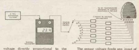
voltage directly proportional to the absolute temperature (°K). The output voltage obeys a linear relationship with temperature and is equal to 10mV/°K. On board calibration circuitry provides an accuracy of 1°K.
