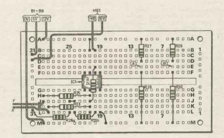
Fig. 12.4. The layout of the components on the Verobloc for the circuit in Fig. 12.3.
