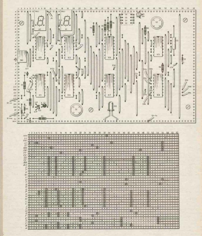
Fig. 5. Stripboard component layout. Note that the 8-pin d.i.l. switch (S3 to S6) is mounted on the copper track side of the board The underside view shows the positions of the track breaks but omits the d.i.l. switch for clarity.
