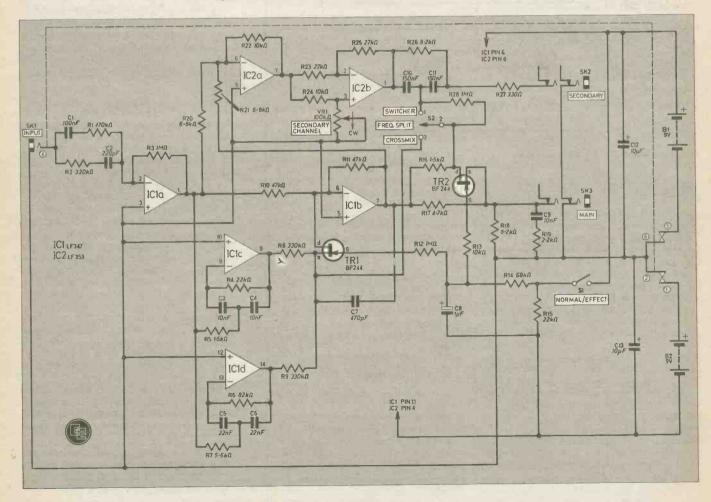
**CROSSMIX mode** is selected thus preyenting bass signals from the main output getting into the secondary output. R27 is included to isolate the output of the op-amp from cable capacitance which could otherwise cause instability.
