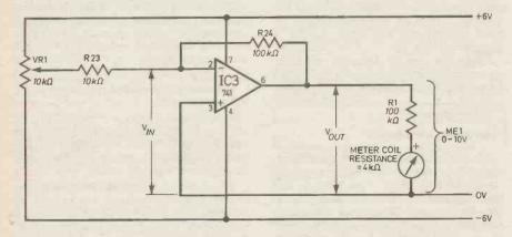
Fig. 12.1. Using an op-amp as an inverting amplifier. Offset null compensation is not essential and is omitted. You could connect up this circuit on *Minilab* and test its action. For positive input voltages from VR1, reverse the connections to the meter.
