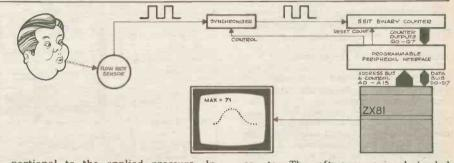
portional to the applied pressure. Internal Hall effect switches in the sensor produce a train of pulses at its output. The pulse rate is thus proportional to the applied pressure.
