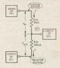
Fig. 12.2. The resistors of the inverting amplifier re-drawn as a potential divider. The current flowing to the (-) input can be ignored as it is very small.
