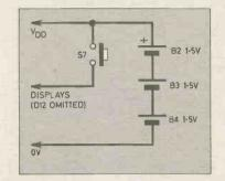
Fig. 4. Optional battery only power supply. The display is enabled with S7.
