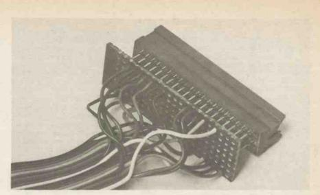
The stripboard/edge connector fully wired. The two outermost connector positions should be fitted with inserts to act as alignment guides.
