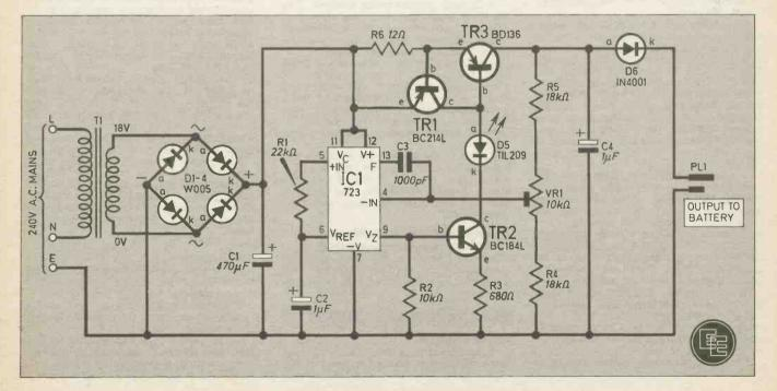
and capacitor C1 provide a smoothed d.c. supply of about 20V. The circuit has to charge the battery on a fixed current until a pre-set full-charge voltage is reached and then maintain this voltage by reducing the current.
