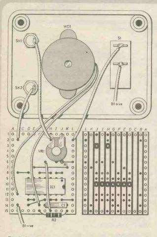
Fig. 2. Stripboard layout and inter-wiring diagram.
