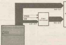
The existing software commands the computer to repeatedly send data to a particular port number, OC. The port number appears on the lower half of the address bus at this time and is de-
