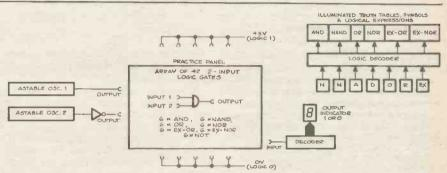
user via sockets on the top panel. A set of jumper leads allow these to be easily interconnected as required. Two pulse generator outputs are provided in the design at similar sockets for feeding clock driven logic circuits, as are
