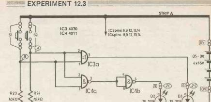
Fig. 12.9. Circuit of a half-adder.
