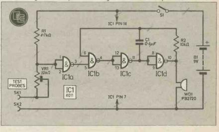
Fig. 1. The complete circuit diagram for the Continuity Tester.
