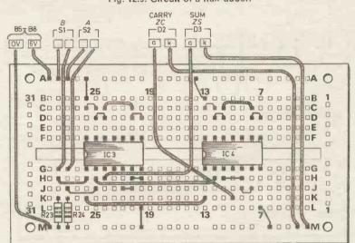
Fig. 12.10. The layout of the components on the Verobloc for the circuit in Fig. 12.9. Unused inputs are connected to 0V or +6V so that the i.c.s operate correctly.
