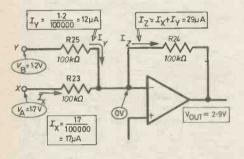
Fig. 12.5. Potentials and currents in the adder when inputs are 1.2V and 1.7V.
