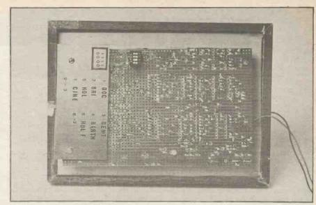
Rear view of the framed Monthly Planner showing the position of d.i.l. switches S3 to S6. An additional board was fixed to the rear of the prototype unit to show the codes for each event (given here as a decimal number). Note the use of the nylon screw in hole *I*/26.
