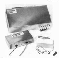
The finished electronic control units. The Power Supply is built into the Control Logic case.
