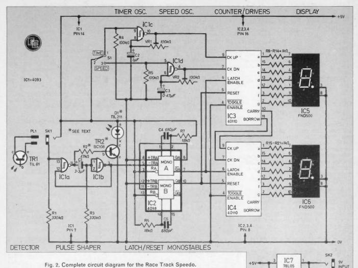
Fig. 2. Complete circuit diagram for the Race Track Speedo.
