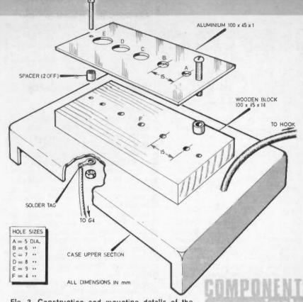
Fig. 3. Construction and mounting details of the locating block and metal mask on the case lid. Increasing the length of the spacers increases the difficulty factor.
