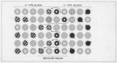
Fig. 3.2. A depletion region forms at a pn-junction.
