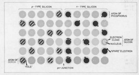
Fig. 3.1. Part of a crystal of silicon doped as p-type on the left and as n-type on the right (very diagramatic).
