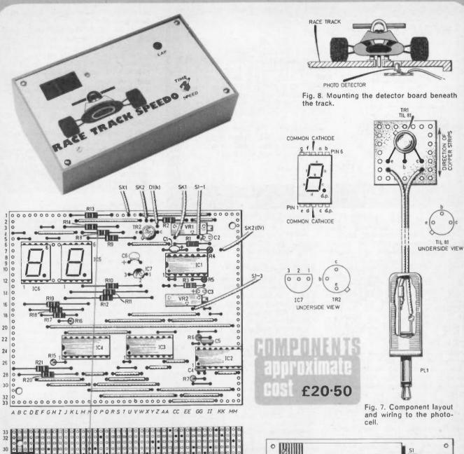
Fig. 4. Component Layout and details of breaks to be made on the underside of the circuit board.
