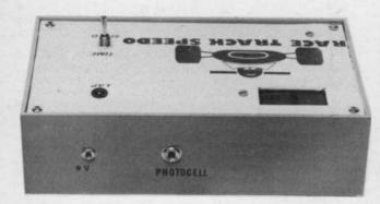
These holes are to suit the 3.5mm and the 2.5mm jack sockets and are 6mm and 4mm diameter respectively.
