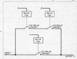
Fig. 8.7 A relay (switch) realisation of the logic module in Fig. 8.6.
