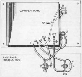
Fig. 6. Interwiring details from the board to the front and back panels.
