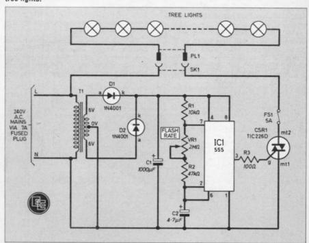
comes to approximately 3Hz. For the slowest flash rate we must do the calculation with VR1 at its maximum resistance of  $2M\Omega$  and this gives approximately  $0\cdot074\text{Hz}$  which works out at about four flashes a minute.
