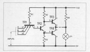
Fig. 8.5 A TTL 3-input NAND gate. This requires a special type of transistor having in this case three emitters.
