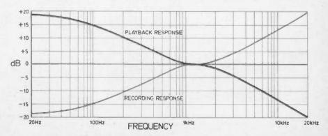
Fig. 1. Playback and recording responses for a hi fi magnetic cartridge input (RIAA).
