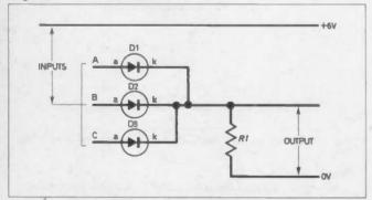
Fig. 8.1 A 3-input OR gate constructed using diodes.
