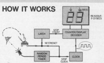
When the period produced by the RANDOM PERIOD TIMER has elapsed, the i.e.d. lights up. At the same time the CLOCK is turned on and its output pulses reach the COUNTER. The end of the time period also sets the LATCH which enables the counter, so the number of clock pulses it receives are displayed on the read-out. Pressing the STOP button resets the latch which freezes and displays the count so far.
