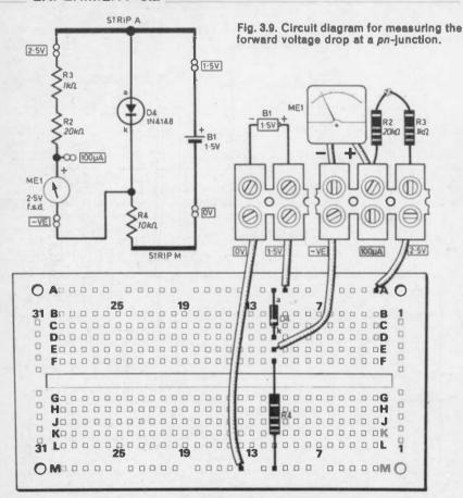
Fig. 3.10. The layout of Fig. 3.9 on the breadboard.
