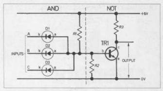
Fig. 8.3 A 3-input NAND consisting of a 3-input AND followed by a NOT gate.
