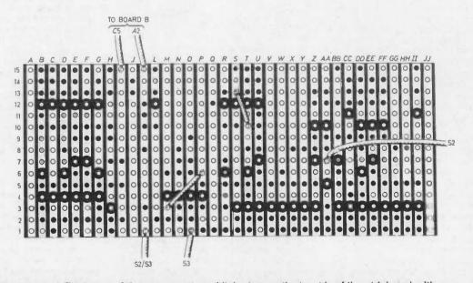
Fig. 2. (upper) The layout of the components and link wires on the topside of the stripboard with wiring to opto devices. Note that some link wires share a locating hole; (lower) the breaks and connections to be made on the track side of the stripboard.
