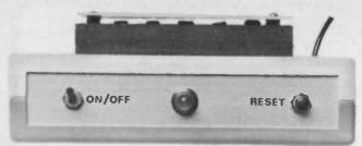
Face view of the completed prototype. You can see the metal mask panel sitting above the wooden locating block on the case top.
