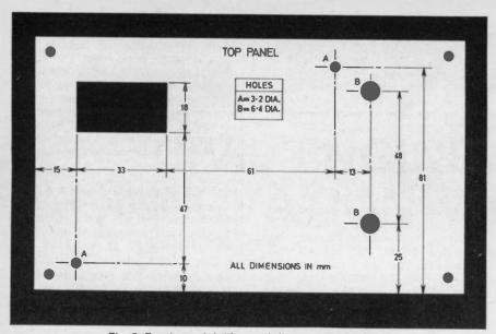
Fig. 5. Front panel drilling and display cut-out details.
