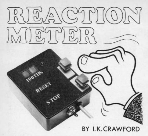
THE Reaction Meter is a device to measure the speed of a person's response to stimulation of the optic nerve by monitoring how fast one can react to an l.e.d. lighting after a random period of time has elapsed.
