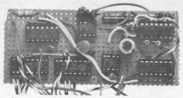
Close-up view of the completed prototype main circuit board.
