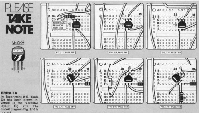
In all Experiments in Part 2, the vMos transistor has been drawn with its flat face on the wrong side. If this is placed in the Verobloc layouts as shown, the Experiments will fail to work. Of particular importance is Expt. 2.1, Fig. 2.7. If wired as shown the l.e.d. will be destroyed. Modifications for the appropriate section of each Verobloc layout for Part 2 Experiments appears above. All circuit diagrams are correct.
