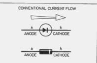
Fig. 3.6. The symbol used for a diode in circuit diagrams and the way diodes are marked (in EE projects) to show their polarity.
