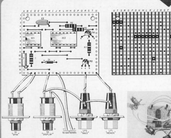
Fig. 2. Stripboard component layout and interwiring diagram. The track breaks on the underside of the board are also shown.
