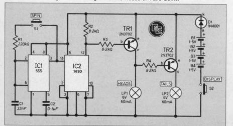
The power for the circuit is supplied by four 1.5V batteries, diode D1 being included to drop the six volts from the batteries down to suit the 7490 TTL i.c.
