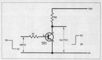
Fig. 8.2 A translator in the grounded emitter mode will produce a NOT gate.
