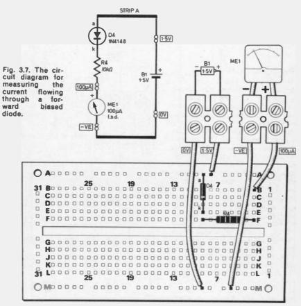
Fig. 3.8. The layout on the breadboard for the circuit in Fig. 3.7.
