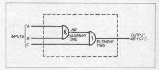
Fig. 8.6 The gate arrangement in the dotted box is known as a "logic module".
