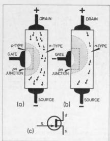
Fig. 3.12. Schematic diagram of an n-channel junction field effect transistor (f.e.t.) (a) gate at 0V (b) gate at -ve potential (c) circuit symbol.
