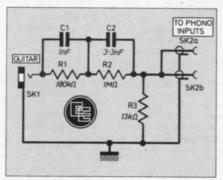
Fig. 2. Circuit diagram of the Guitar Adaptor.
