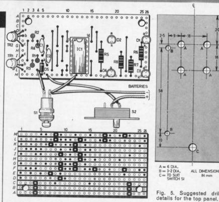
Fig. 3. Component layout, interwiring and details of breaks on the underside of the stripboard.
