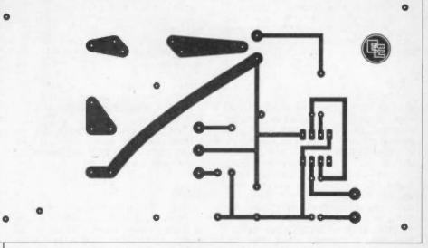
Fig. 2. Full size master of the printed circuit board.
