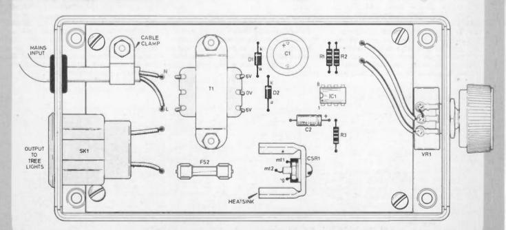
Fig. 3. Component layout of the p.c.b. shown mounted in the case with all interwiring shown.
