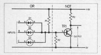
Fig. 8.4 An OR gate followed by a NOT produces a NOR gate.
