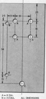
B = 3-2 DIA. C = TO SUIT SWITCH SI N mm Fig. 5. Suggested drilling
