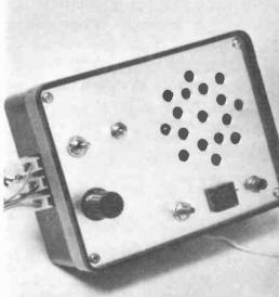
The Master unit showing front panel controls and the terminal block to the left of the unit.
