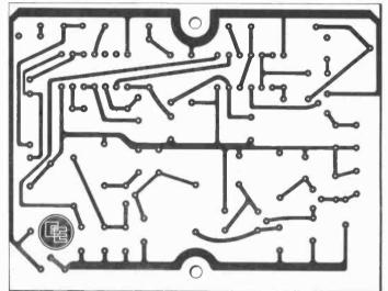
Fig. 4. The layout of the components on the top side of board A and connection details to board B. Lower diagram shows full-size master of the p.c.b. pattern for this board.
