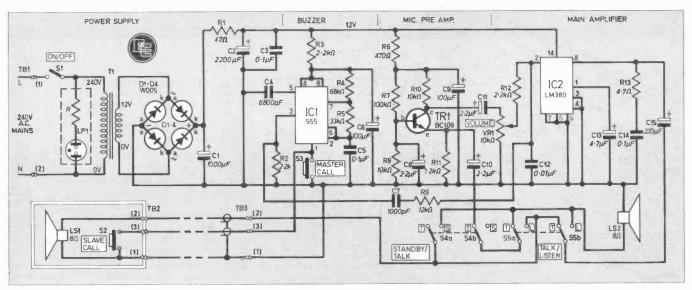
Fig. 1. Full circuit diagram of the Intercom. The circuit of the Slave unit is shown in the inset bottom left
