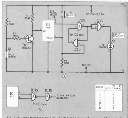
Fig. 7.7a. Light triggered counter, (b) decoding two outputs to light the l.e.d. when a count of 40 is reached.
