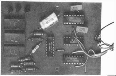
Close-up view of the two prototype printed circuit boards with all components in position.
