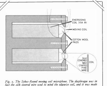
rigid by the wax with which it was impregnated while winding it between
