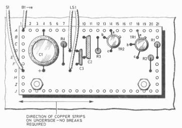
Fig. 2. The layout of the components on the circuit board and interwiring of the remainder of the components mounted in the case.
