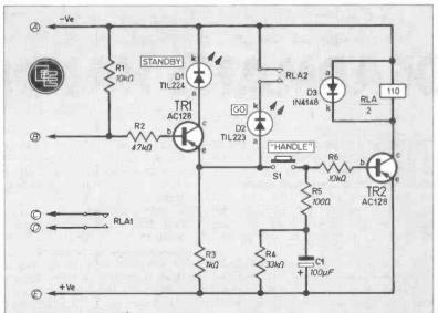
connection that leads to the output terminals and Fig. 2. Full circuit diagram of the Model Railway Deadman's Handle. Points point E the other terminal.
