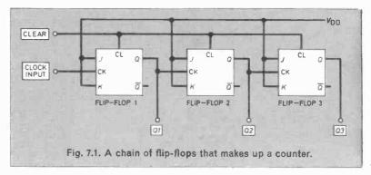
high to low (the negative-going edge of a pulse). A high pulse on the clear (or reset) line forces all Q outputs to low (0) and all  $\overline{Q}$  outputs to high (1).
