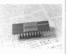
Finally there is a digital to analogue converter to convert digitally synthesised speech into an audio signal
