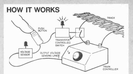
A transistor controlled switch is connected in series in the controller track output.
