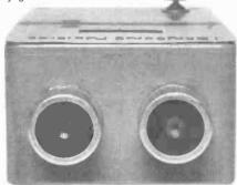
Close-up view of the transducers squarely mounted on the outside of the case.
