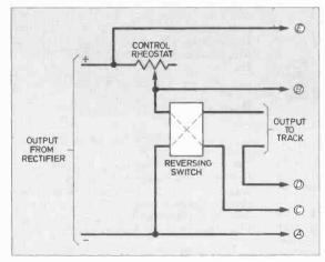
Fig. 1. Interior schematic of part of the train controller showing connection points. Some models may not have a reversing switch so follow back connections from output terminals for points  $\mathcal G$  and  $\mathcal D$ . Some control rheostats may have only two terminals. Point  $\mathcal B$  is the connection that leads to the output terminals and point  $\mathcal E$  the other terminal.
