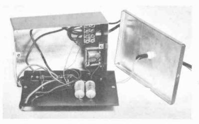
Interior view showing board displaced. The transformer and underside of the component board can be clearly seen.
