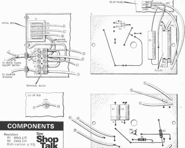
Fig. 2. Interwiring details. Topside of the board is seen at the top of the page with underside below.
