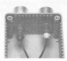
Phono connections to the transducers securely glued to the case.
