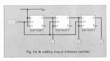
If Q1 and Q2 are both low, the next pulse changes Q1 to high, but Q2 remains unchanged as its J and K inputs were both low at the instant of change. We go from 00 to 01.
