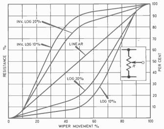
Fig. 1. Potentiometer "laws", connecting the amount of wiper movement with the amount of resistance change.
