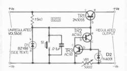
current paths out. It causes the latch formed by TR2 and TR3 to operate when the voltage across VR1 attains approximately (0.55+0.6)V and then isolates the latch from VR1 so current from TR2 collector goes only into the base of TR1.
