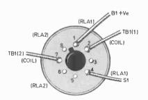
Fig. 2a. Shows the connections to the base of the specified relay.
