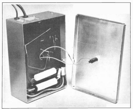
Interior view of the unit showing mounting position of CSR1, circuit board, and reed operating coil.
