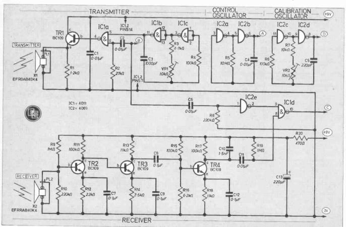
being reduced in duration to 0.2ms via the R8 and C6 coupling network and then being inverted by IC2e. The output is connected directly to the NAND gate IC1d.
