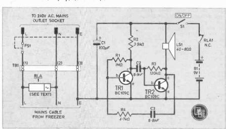
Fig. 1. The complete circuit diagram of the Freezer Alarm.
