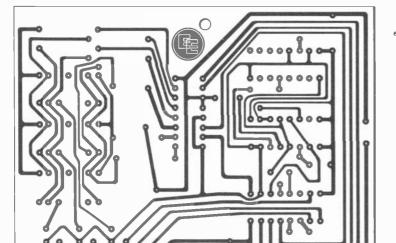
Fig. 5. The layout of the components on board B. The lower half shows the full size pattern required on the underside of board B.
