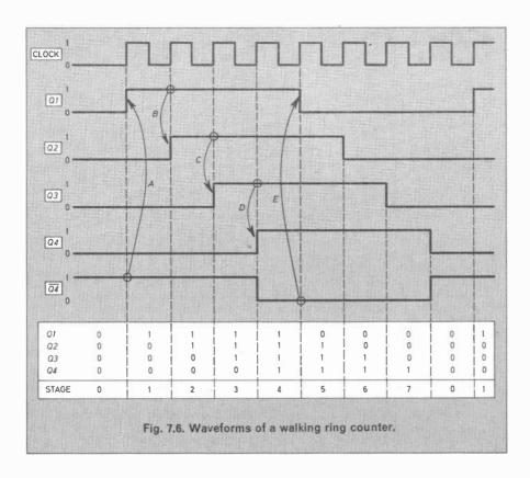
flip-flops are fed to logic circuits that decode them to produce outputs of a different form. We have already mentioned the 1-of-10 and 1-of-8 decoded outputs from the 4017 and 4022 walk-
