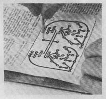
(f) Pricking through the pad centre points onto the copper board.
