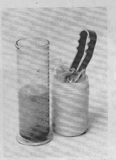
(q) Making up a solution of ferric chloride in a measuring cylinder.
