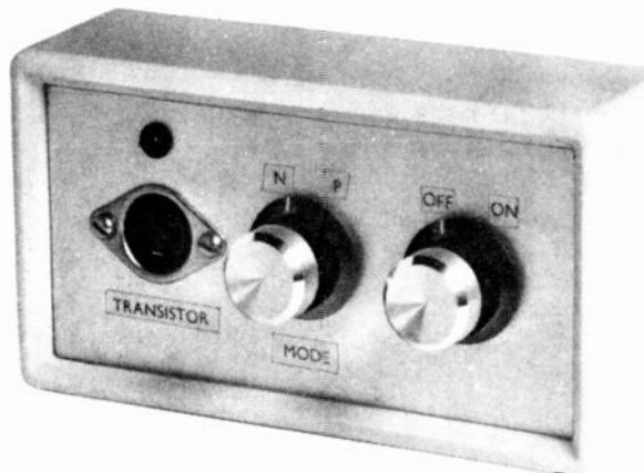
Completed tester showing front panel layout.
