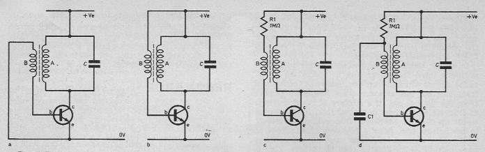
Fig. 5.7. Four ways of connecting our coil into a transistor circuit. The first (a) will not work as there is nothing to turn the transistor on. In (b) the transistor is turned on too much, whereas although (c) is satisfactory, the a.c. current is impeded. By adding a capacitor as in (d) this problem is solved.
