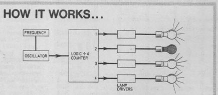
The variable frequency oscillator produces a train of square wave pulses suitable for inputting to a TTL logic section which acts as a divide by 4 counter with four independent outputs. The state of each output (high or low, logic 1 or 0) is dependent on the number of pulses received from the oscillator.
