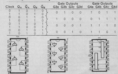
Pin and internal details of the three logic i.c.s employed in the Chaser Light Display.
