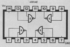
Pin configurations for the CD4001AE.
