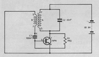
Fig. 5.8. The final circuit we use. This is constructed using the NPN module and the homewound coil. Note the connections to the coil. To check that it is working the VOLTAGE INDICATOR may be used.
