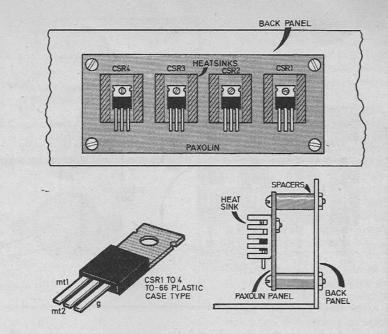
Fig. 3. Details of the triac mounting arrangement and heatsink fittings. Also shows pin configuration for the specified triacs.
