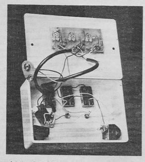
Interior view showing the circuit board mounted on the lid. The positioning of the switches, sockets and light emitting diodes can be seen.
