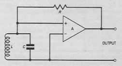
Fig. 5.5. A simple oscillator circuit. The circuit is tuned by the combination *LC* circuit.
