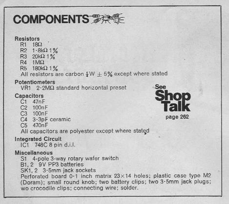
this and SK2 on the right. Both sockets are 3.5mm jack types and require a 6mm diameter mounting hole.
