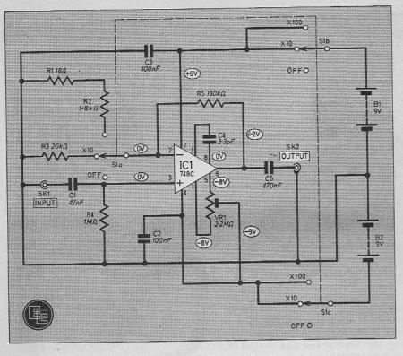
Fig. 2. The complete circuit diagram of the A.C. Meter Converter.
