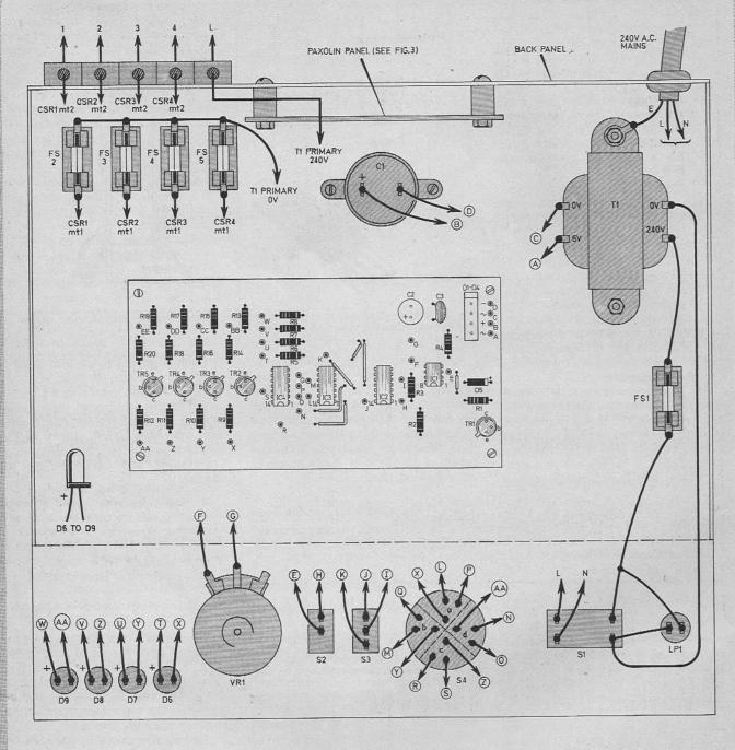
Fig. 4. The layout of the components and board within the case and complete wiring up details of the main unit.
