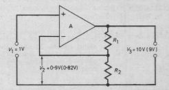
Fig. 5.10. By adding two resistors as a potential divider, the op-amp can have any gain as desired.
