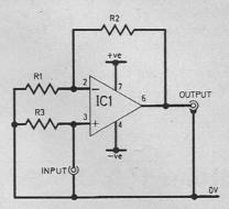
Fig. 1. The basic non-inverting amplifier circuit.
