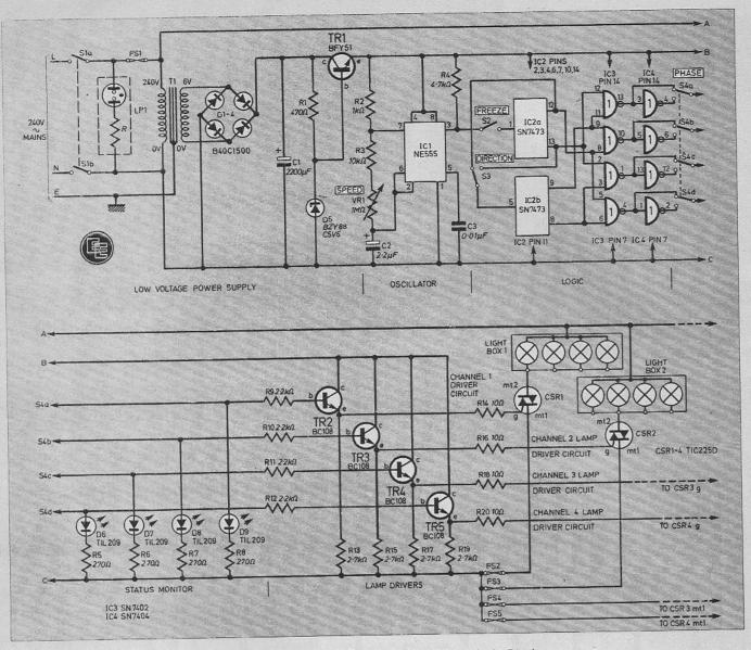
Fig. 2. The complete circuit diagram of the Chaser Light Display.
