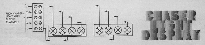
Fig. 5 Light box wiring details to the main unit.
