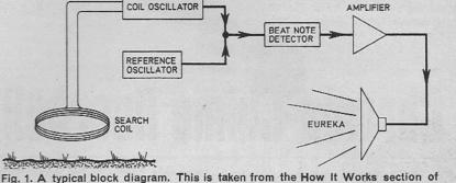
Fig. 1. A typical block diagram. This is taken from the How It Works section of the Treasure Locator (October 1977 Issue—back issues not available)
