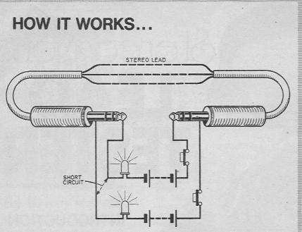
The Stereo/Mono Lead Tester is basically a three-position continuity checker. When a lead is plugged in and one of the switches is pressed the l.e.d. corresponding to that switch should light. If it does not then it would indicate that the lead is open circuit.
