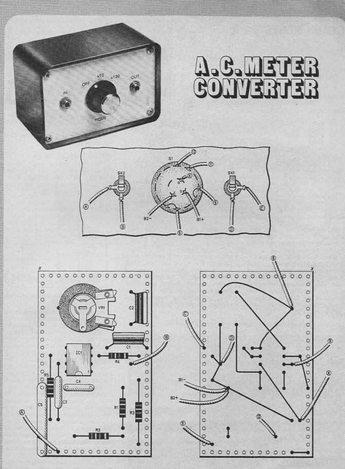
Fig. 3. Component layout and wiring for the plain perforated board. The wiring for the front panel components S1, SK1 and SK2 are also shown.
