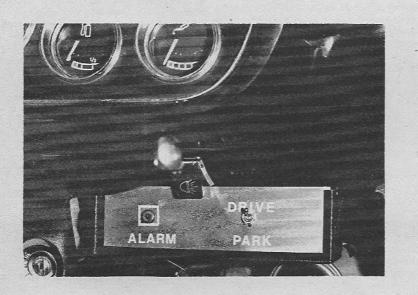
operated the l.e.d. is still lit, but the alarm tone should stop. Now when the ignition lead is applied to the positive terminal of the battery, the l.e.d. should dim, and the alarm bleep should sound again. When S1 is restored to the DRIVE position the tone bleep will stop and the l.e.d. remains unlit.
