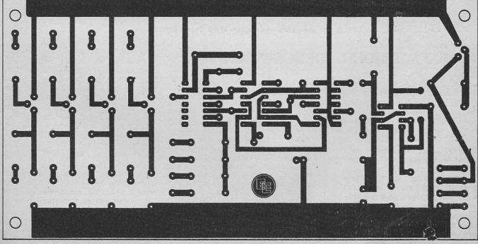
Fig. 1. The copper pattern to be etched on the Chaser Light Display component board, shown full size from copper side.
