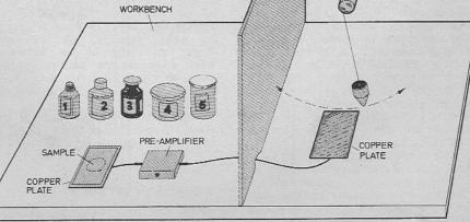
Fig. 2. The various parts of the Radiaesthetic Amplifier
