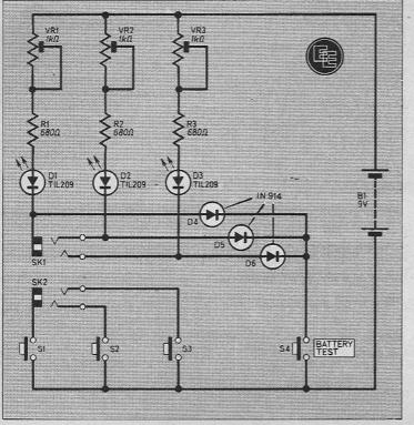
Fig. 1. Circuit diagram of the Stereo/Mono Lead Tester
