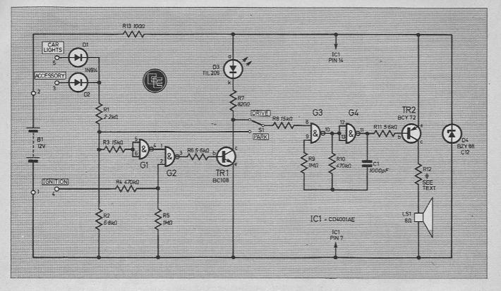
Fig. 2. Complete circuit diagram of the Car System Alarm.
