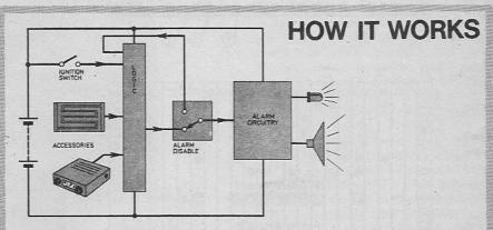
Normally the voltage from the ignition switch when switched on, is at a "high" logic level. This condition when applied to the logic circuitry inhibits the alarm. Basically the logic circuitry is a NOR gate. This means there is no output when *either* the ignition *or any* of the accessories are on.
