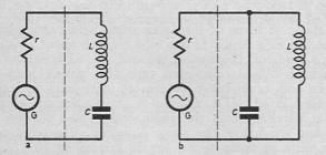
Fig. 5.4. Two ways of connecting an inductor and a capacitor. The first is in series, the second in parallel.
