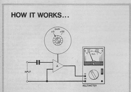
The A.C. Meter Converter is basically an a.c. amplifier with a switched gain of either 10 or 100. The gain being selected by varying the ratio of two resistors. Thus the set-up can be used to measure low level voltages which would be imperceptible using a standard multimeter alone.
