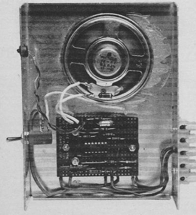
Interior view of the unit showing positioning of components.
