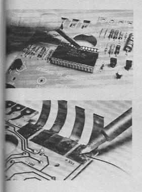
The above photos are reproduced from the Chroma-Chime assembly Manual. *Top:* Breaking off the i.c. socket retaining strips after wiring has been completed. *Bottom:* Soldering the battery contacts onto the p.c.b.
