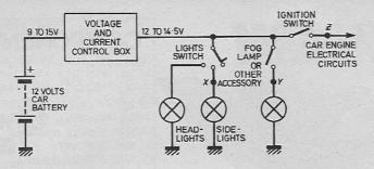
Fig. 1. A typical car electrical system.
