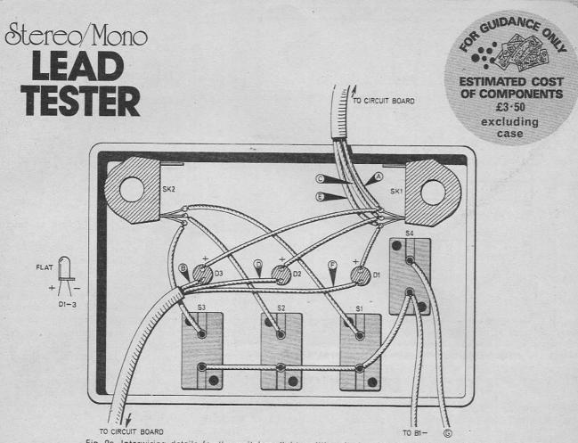
Fig. 2a. Interwiring details for the switches, light emitting diodes (i.e.d.s) and stereo jack sockets.
