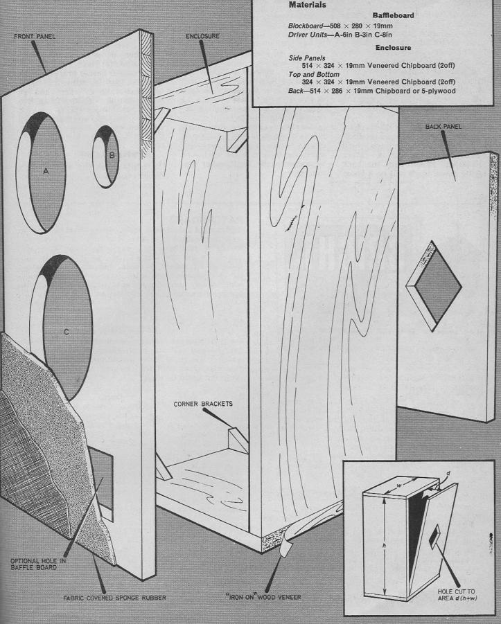
Fig. 1. Constructional details for a low cost loudspeaker enclosure. The method of working out the size of hole required to "tune" the enclosure for best response is shown inset.
