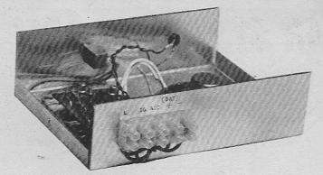
Rear view of the unit showing the mounting of the terminal block for connecting to the car wiring.
