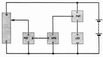
Fig. 3.8. Using the transistor modules to prove that a much reduced current may be used to light the LED.
