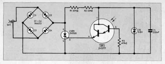
Fig. 1. Complete circuit diagram of the Photoflash Slave Unit.
