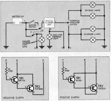
Fig. 6. The complete circult diagram of the Hazard Warning System for both negative and positive earthing systems.
