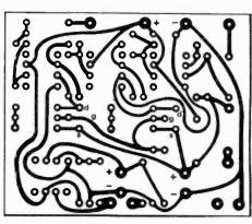
Fig. 1. The underside view of the printed circuit board. The black regions show the areas of copper to remain after etching. Shown full size.
