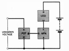
Fig. 3.6. In this experiment we are using an amplifier, driven by a voltage from the POT to light the LED
