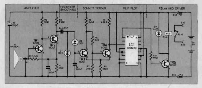
Fig. 1. Circuit diagram of the receiver section of the Ultrasonic Remote Control System.
