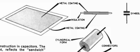
Fig. 3.2. A typical form of construction in capacitors. The symbol shown to the right, reflects the "sandwich" construction of a capacitor.
