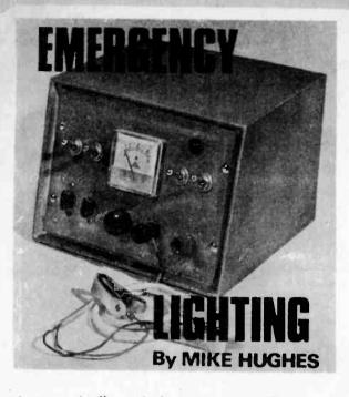
Automatically switches on an auxiliary lighting system when mains supply fails
