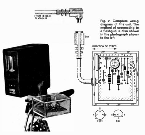
Three extra rows of holes are provided on the component panel so that there is space for mounting holes to be drilled, should it be necessary to bolt the panel to the case. It was not in the case of the prototype because the panel was found to be a firm fit into the housing.
