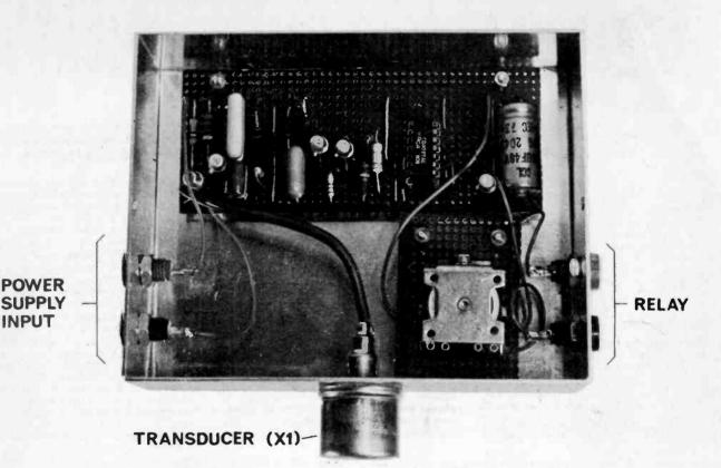
Interior view of the receiver showing positioning of component board, relay, transducer and sockets.
