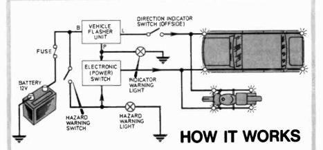
To obtain the "Hazard Light" effect the direction indicator is switched to the offside position, i.e. right turn. This completes the circuit to the flasher unit via the offside lights thereby turning them on and off in the normal manner. At the same time the P output from the flasher unit supplies a pulsating voltage which turns the vehicle's indicator warning light on and off.
