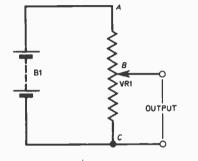
Fig. 3.3. Circuit symbol for a variable resistor. The zigzag line represents the *track*, the arrow head the *wiper*.
