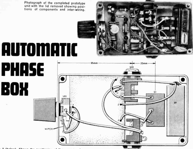
Fig. 2 (below). Shows the positioning of the components on the topside of the printed circuit board.
