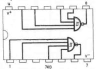
Fig. 7.6. Pin connections of the 7413 four-input Schmitt NAND.
