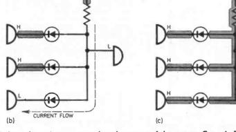
Fig. 7.3.(a) An AND gate using three diodes and a resistor connected to the output of three gates. Gates A, B, C and D can be any type of gate. (b) Current flow when the output of one of the gates is low (c) State of the circuit when the output from all gates are high.
