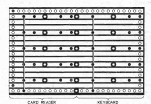
Fig. 7.12, Layout of the card reader (left) and keyboard (right) on the 0.15in matrix stripboard. Note the cuts in the strips under the board. The board can be sawn in half if the two units are to be used separately.
