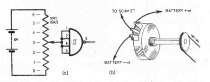
Fig. 7.9.(a) The input to the Schmitt can be from a potentiometer connected across a 6V battery. The potentiometer can be part of a working model as shown in (b).
