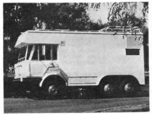
Mini-Mobile OB van introduced by Marconi last year. Note the cameraman with his hand-held portable camera protruding through the vehicle roof.
