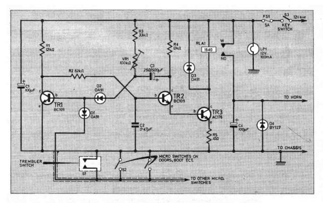
Fig. I. The Complete circuit diagram of the Car Burglar Alarm.
