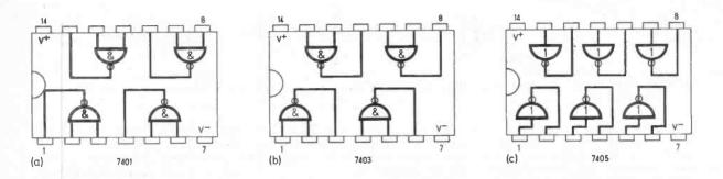
Fig. 7.4. Pin connections for three types of open collector i.c.s. (a) the 7401 quad two-input NAND gate (b) the 7403 quad two-input NAND gate and (c) the 7405 hex INVERTER.
