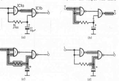
Fig. 7.1. Single pulse generator (a) shows the circuit before it is activated. The shaded areas indicate a high level. (b) shows the state of the circuit just after the input has gone high (c) shows the state after the capacitor has had time to charge and (d) shows the circuit when the input returns to low.
