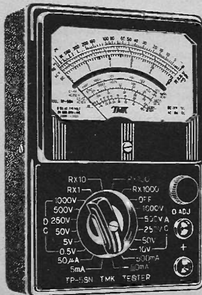
Left the TMK model TP5SN 20,000 \Omega/\text{V} meter and right a Russian meter having a similar sensitivity. Both these meters are suitable for use with our projects and for the checks described above.
