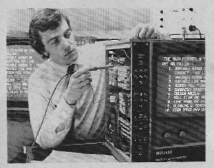
An engineer works on a visual display unit which employs MOS memory chips.
