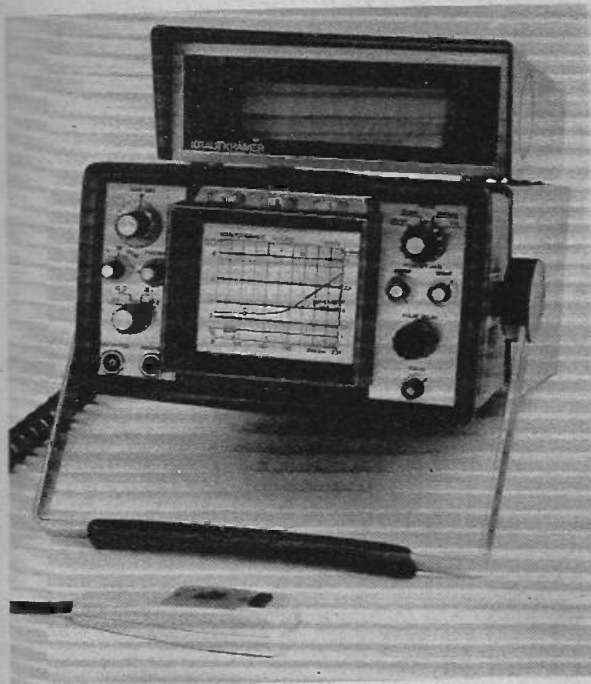
The Wells-Krautkramer ultrasonic flaw detector which can examine steel from depths of 10mm to 5m. A recorder is shown at the top.
