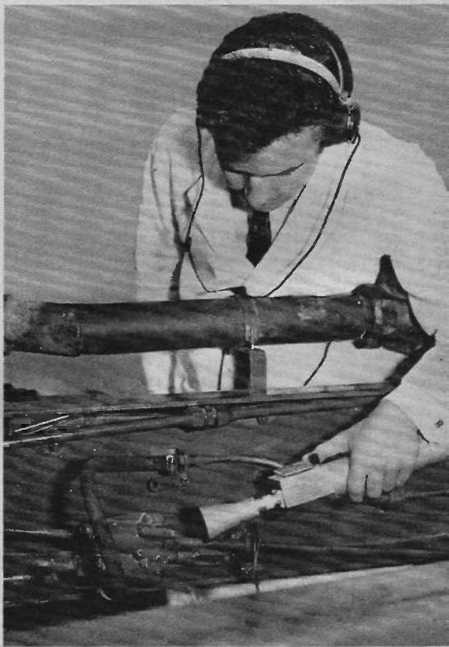
The Dawe Instruments ultrasonic leak detector shown in use.
