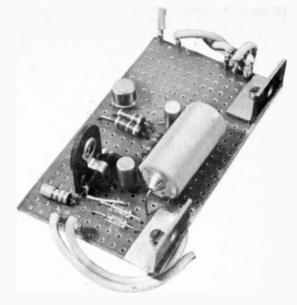
Photograph of the circuit board for the Baby Snatch Alarm.
