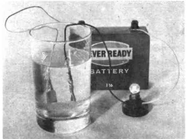
Fig. 2.2. Adding table salt increases current flow and the bulb glows more brightly.
