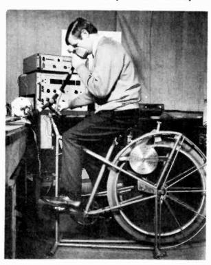
Using a Transfer Function Analyser to determine the relationship between respiration and work done by humans. (Solartron Electronic Group Ltd)
