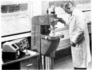
Checking the finish of a lens with the Talyrond 73 roundness measuring system. This system which can detect surface irregularities of the order of one millionth of an inch, uses a special purpose computer to correct for inaccuracies in work positioning etc. Defects of the work plece are recorded on a rotating chart. (Rank Precision Industries Ltd.)
