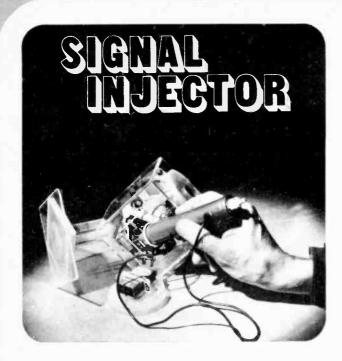
The photograph on the left shows the completed signal injector being used to test the Astron receiver. Complete test procedure for the Astron is given in the text of this article. The injector can also be used with other radios and audio equipment.
