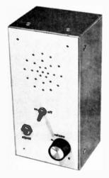
Fig. 5. A completed case of a small amplifier showing holes drilled for loudspeaker
