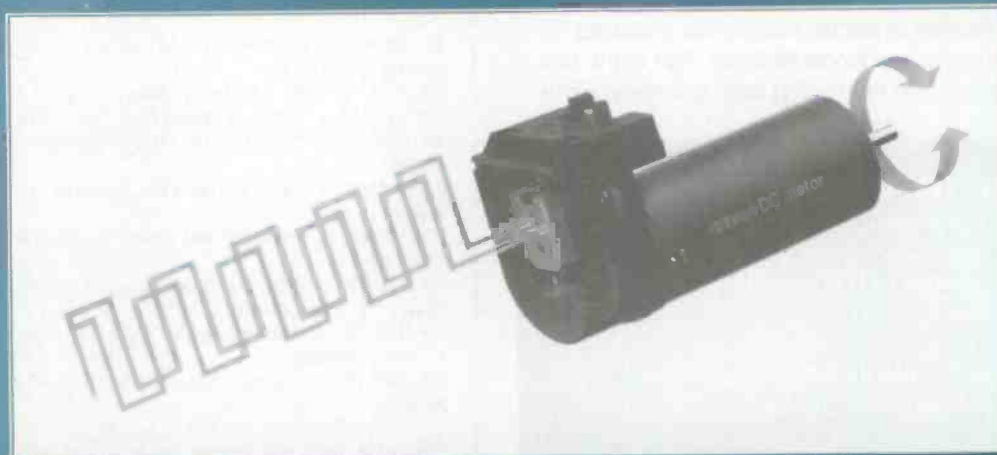
Figure 13: Output signal of servo potentiometer as a function of rotational position.
