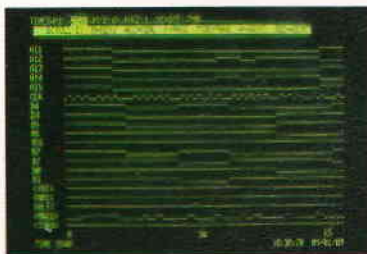
A Z80 logic trace, showing part of the test sequence
