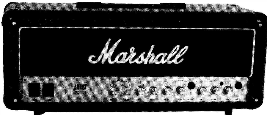
The Marshall Artist 3203, a 30W amplifier which has a valve output stage and an IC preamplifier. Note the 'standby' switch, a common feature on valve amplifiers. The 3203 has only one input channel but two tone control networks. This allows the user to set both a 'backing' sound and a brighter 'solo' sound and to select between the two in performance using a foot-switch.
