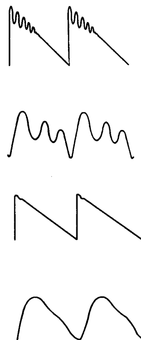
Fig.5 VCF response. From top to bottom: high frequency, high Q (resonance control clockwise); low frequency, high Q; high frequency, low Q (resonance control anticlockwise); low frequency, low Q.
