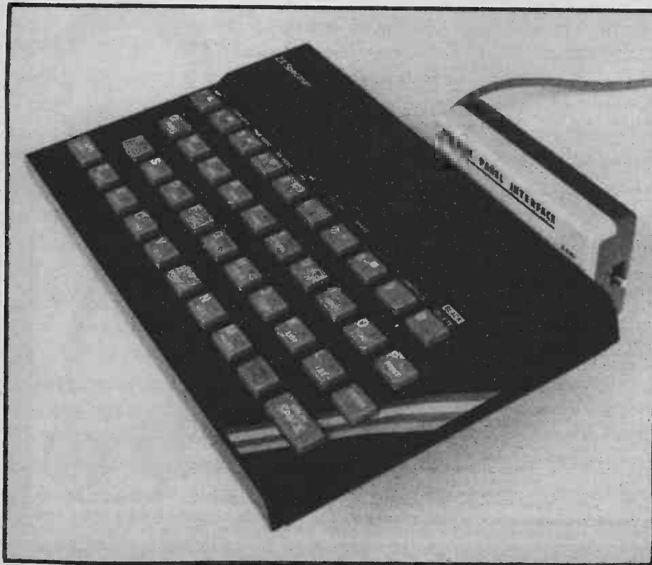
Like all good add-ons for the Spectrum, our interface simply plugs onto the expansion port.
