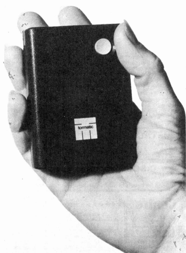
Fig 9. This small hand-set is the control for radio-controlled garage doors.
