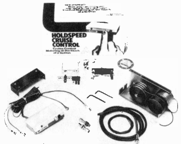
Fig 4. Retrofit cruise control is possible with this kit. The right chain-coupled unit stores the throttle position required. It is operated by the left-hand push button unit. The brake pedal electric connection is used to cancel the position during deceleration.
