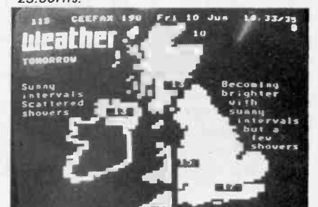
The weather map is just one example of a rolling page. Although always page 115, this page alternates between two displays, this is page B (may just be seen top right).
