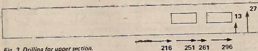
Fig. 3. Drilling for upper section.
