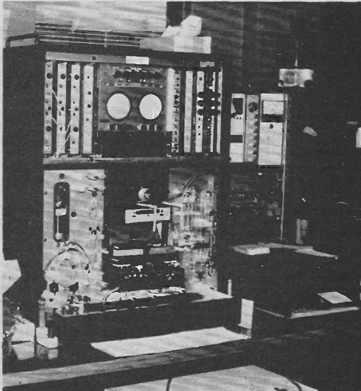
Fig. 7. Multiparameter Model S Coulter Counter with covers removed.
