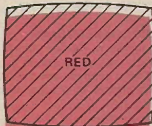
Fig. 48. Purity adjustment is done with the red gun only working. With the scan coils pushed fully forward, the purity rings are used to position the beam deflection-centre horizontally and vertically, to obtain central red spot as in (a). The scan coils are then brought backwards sufficiently to obtain a pure raster as in (b).
